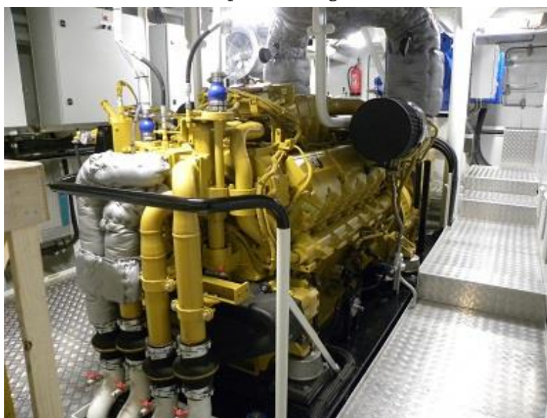
Aft Caterpillar Main generator
