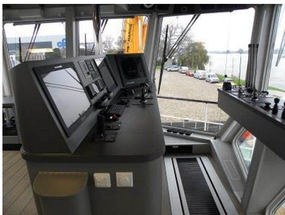
Fore ship Bridge Console
