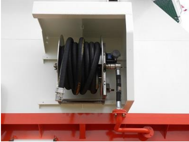
Fuel supply winch
