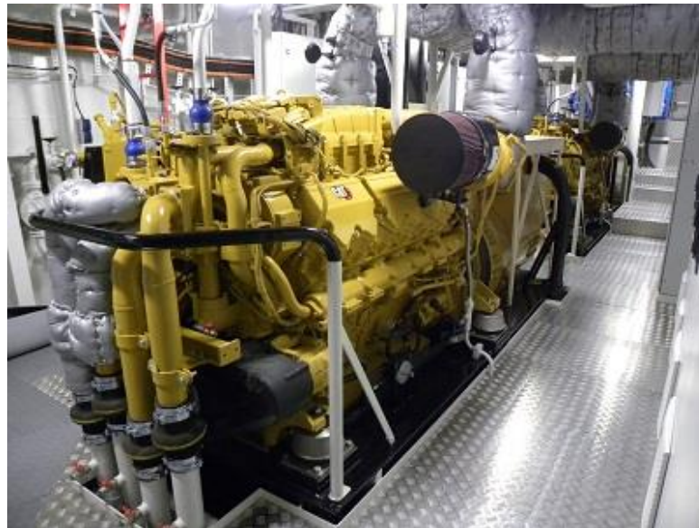
Aft Caterpillar Main generator
